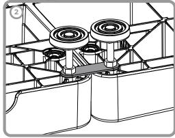
(2) SCREW FEET THROUGH THE LINKING BAR AND TIGHTEN UP SECURELY SO THE THE LOCKING NUT IS FIRMLY AGAINST THE LINKING BAR.
