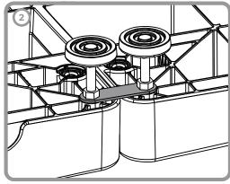
(2) SCREW FEET THROUGH THE LINKING BAR AND TIGHTEN UP SECURELY SO THE THE LOCKING NUT IS FIRMLY AGAINST THE LINKING BAR.
