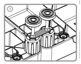
(3) IF USING WITH THE EXTENDING FOOT FEATURE ENSURE THE LINK BAR IS BETWEEN THE BOTTOM OF THE EXTENDING FOOT AND THE LOCKING NUT.
